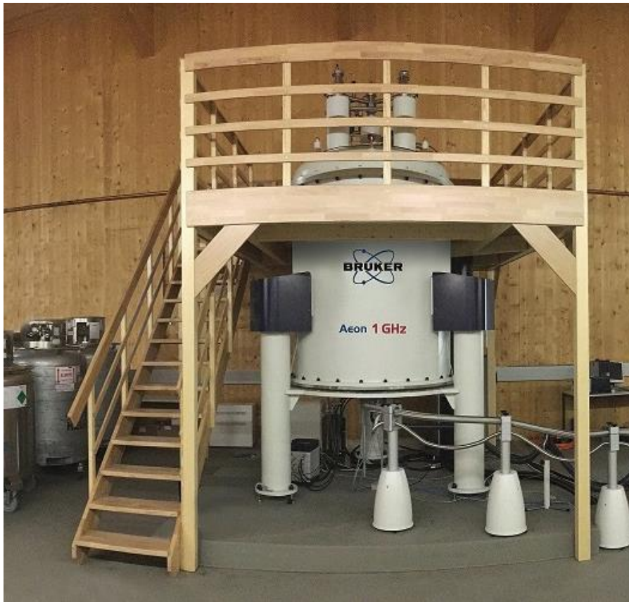
2016: First 23.5 Tesla magnet (1 GHz) Bayreuth University, Germany.
