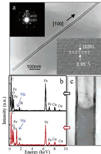
**Figure 3.** (a) Low-magnification TEM image of an  $\text{Fe}_3\text{O}_4$  nanotube, with the SEAD shown in the upper inset. (Lower inset) HRTEM images taken on the tube wall. (b) EDS spectra of solid (black curve) and hollow (red curve) part of a partial etched  $\text{Fe}_3\text{O}_4$  nanotube (c).
