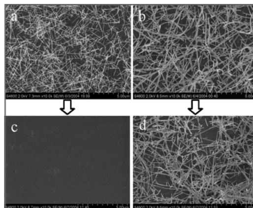
**Figure 2.** SEM images of MgO nanowires before (a) and after etching (c); MgO/Fe<sub>3</sub>O<sub>4</sub> core-shell nanowires before (b) and after the same etching process (d).
