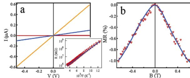
**Figure 4.** Electrical measurements of individual  $\text{Fe}_3\text{O}_4$  nanotubes. (a)  $I$ - $V$  curves taken at three different temperatures of 290 K (orange), 180 K (blue), and 77 K (red). (Inset) Arrhenius plot ( $\log R \approx 1/T$ ) and its linear fitting (blue line). (b) MR measurement at 77 K. Data points are depicted as the red triangles with the blue curve as a guide for the eyes.
