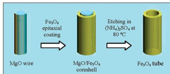
**Figure 1.** Schematic illustration of the fabrication process of Fe<sub>3</sub>O<sub>4</sub> nanotubes.
