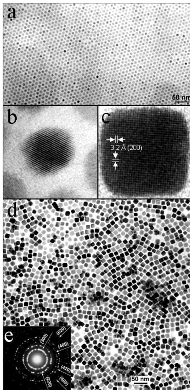
**Figure 1.** (a) Transmission electron micrograph (TEM) image of spherical PbTe NCs (monolayer assembly); (b) HRTEM of a spherical PbTe NC; (c) HRTEM of a cubic PbTe NC; (d) TEM image of cubic PbTe NCs (monolayer assembly); (e) SAED of cubic PbTe NCs ( $\sim 40$  NCs).
