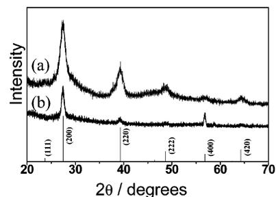
**Figure 2.** X-ray powder diffraction patterns of (a) spherical PbTe NC (8 nm in diameter) assembly on Si wafer; (b) cubic PbTe NC (14 nm in size) assembly on Si wafer.
